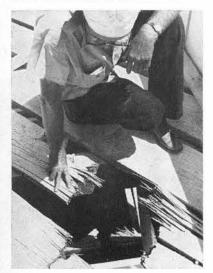
HOLE CAUSED by direct hit on water target by 500 lb. nonexplosive bomb is examined by D. S. Cain. Instead of explosives, bombs carried electronic telemetering instruments. Drop tests were conducted almost every day, weather permitting.
